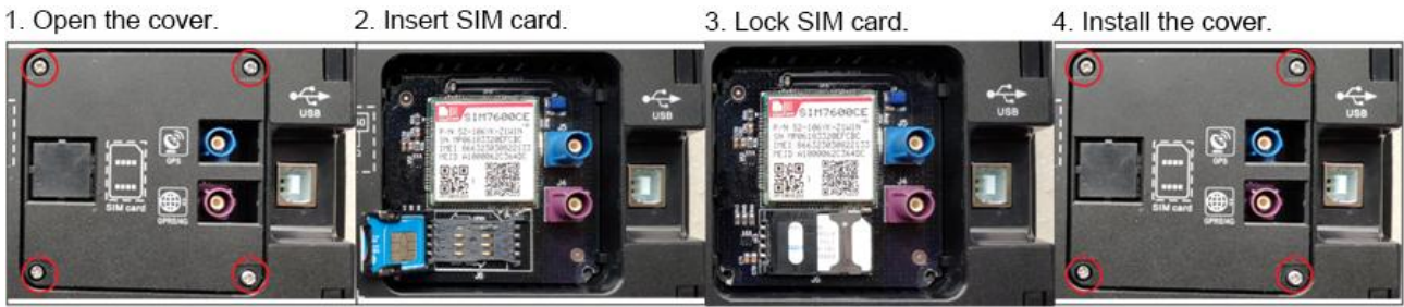
Fig.14 SIM Card Installation Method
