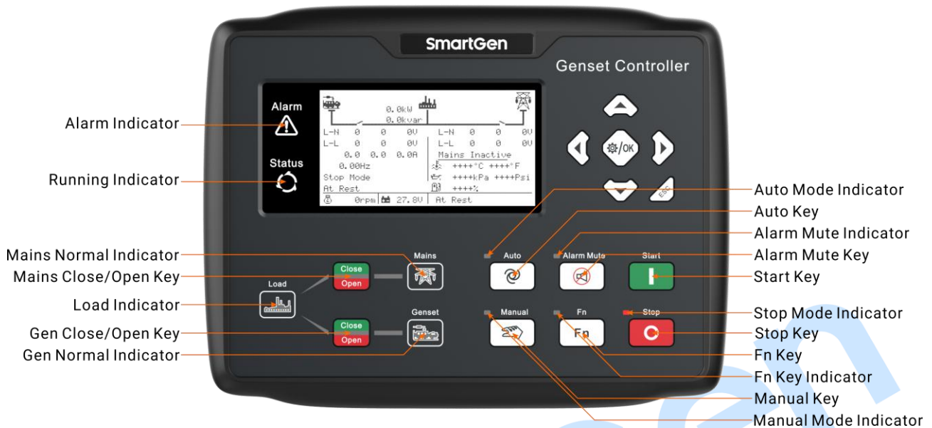
Fig.1 HGM9420N_HGM9420LT Panel Indication
