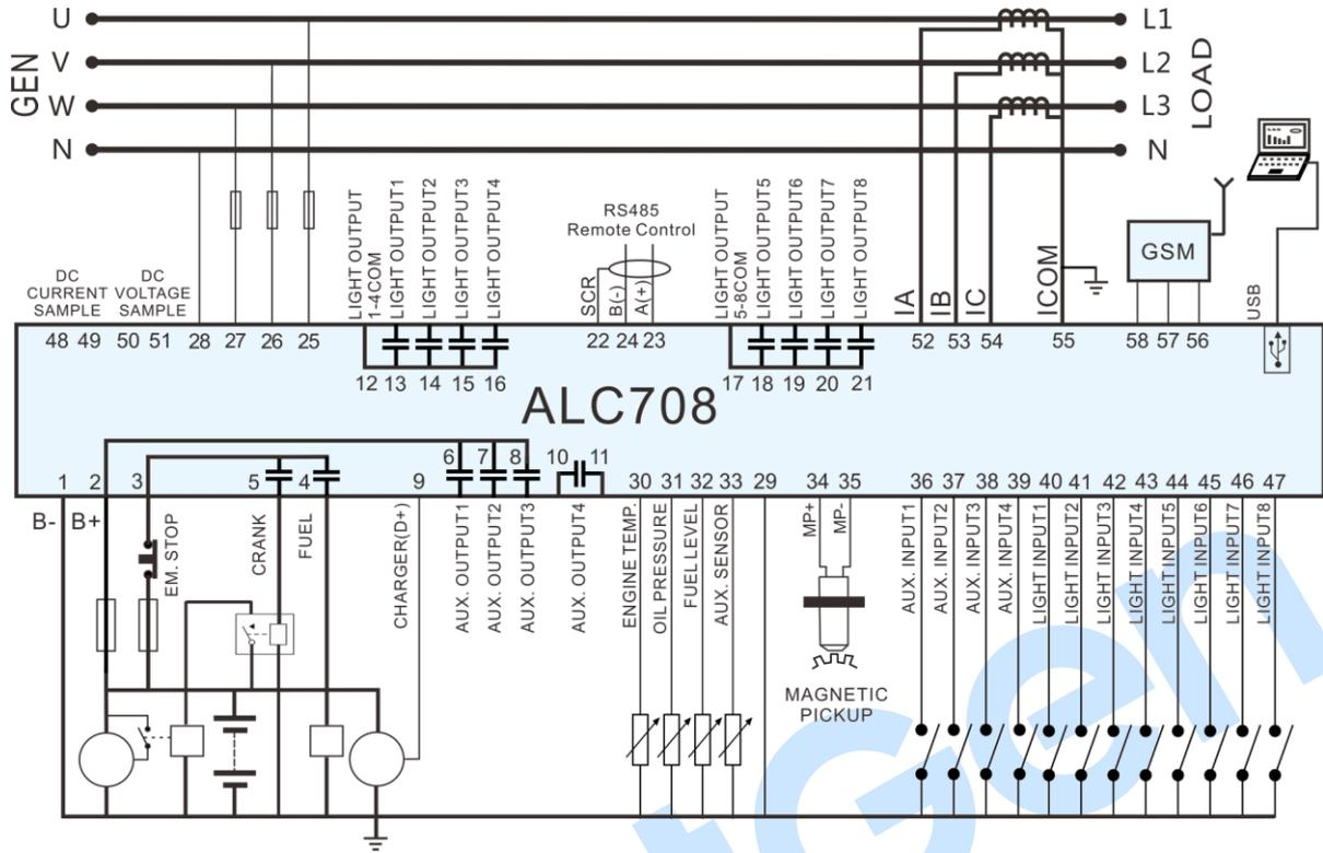
**Fig.4 ALC708 Typical Wiring Diagram**
