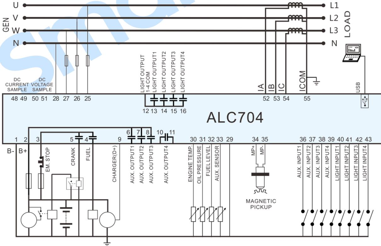
**Fig.5 ALC704 Typical Wiring Diagram**
