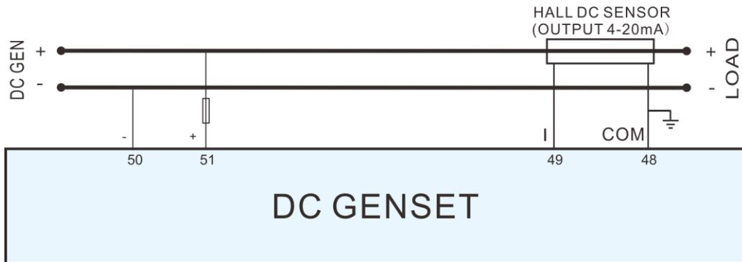
**Fig.6 ALC704/708 DC Generator Typical Wiring Diagram**
